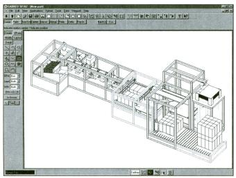
documented for manufacturing and the installation of parts. TECHNICAD performs kinematic analysis for machines with moving parts such as gears, cams, belts and drives as part of the design process. Developing 3D CAD designs and generated detailed engineering layout from the 3D models is an everyday task at TECHNICAD.
